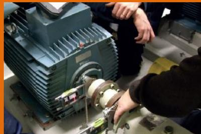
▶ Minimise wear, production stoppages and unnecessary costs with a laser-based shaft alignment tool from FIXTURLASER.
